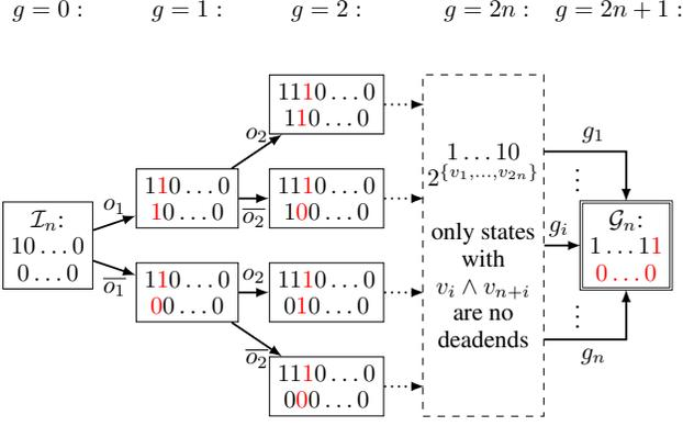
Figure 1: Visualization of the induced transition system of the family of planning tasks  $\Pi_n$ . Nodes represent states where the top row denotes the values of the  $x$  variables in ascending order and the bottom row denotes the values of the  $v$  variables in ascending order.
