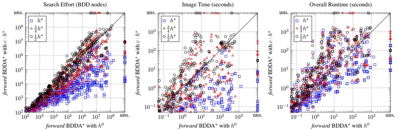
Figure 3: A comparison of *forward BDDA\** with the blind heuristic  $h^0$  and with a given fraction perfect heuristics ( $c \in \{1, \frac{3}{4}, \frac{1}{2}\}$ ) which includes the search effort (left), the cumulative time of the image operation (center) and the overall search time (right).
