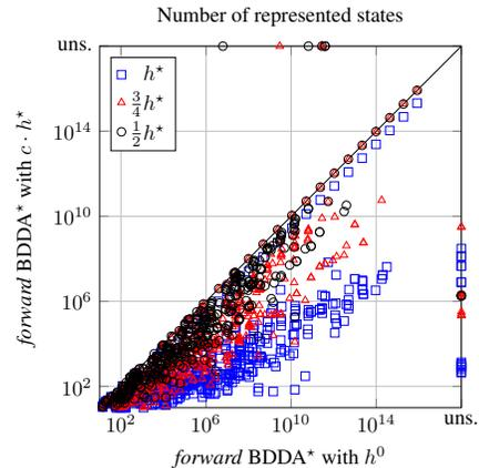
Figure 4: A comparison of the represented (“must-expand”) states of *forward BDDA\** with the blind heuristic  $h^0$  and with a given fraction perfect heuristics ( $c \in \{1, \frac{3}{4}, \frac{1}{2}\}$ ).
